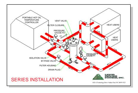
The element is replaced without shutting down the heating system. The inlet and outlet valves are shut off, maintaining flow through the bypass. The filter is cooled and the element removed and replaced with a new one. To re-commission the filter, tighten and torque the top closure plate, open the valves on the filter and purge any air from the housing through the vent valve on top. The filter is now "on line."
