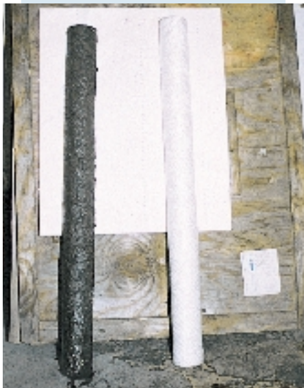
Hot oil filters use cartridges (shown) with excellent dirt holding capacity, and they offer easy disposal.
