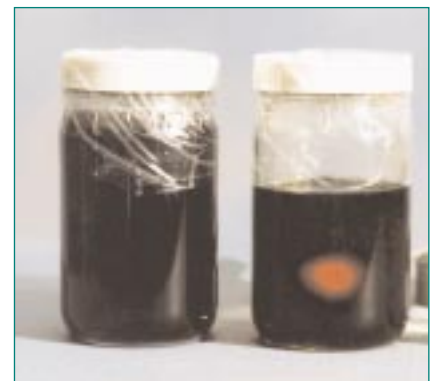
Photo 1. A laser light projected into two samples of heating oil. The unfiltered oil on the left lets no light through; the filtered oil on the right does. The filtration process has improved the oil's viscosity and reduced the particle count.
